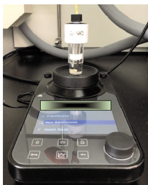
Fig. 20 Anodic oxidation using an ElectraSyn 2.0 apparatus
