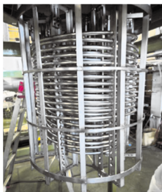
Fig. 17 corrosion-resistant and heat-resistant alloy flow reactor (inner diameter 10 mm)
