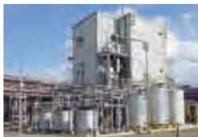
Facility for test production using hydrochloric acid oxidation process (Ehime Works)
